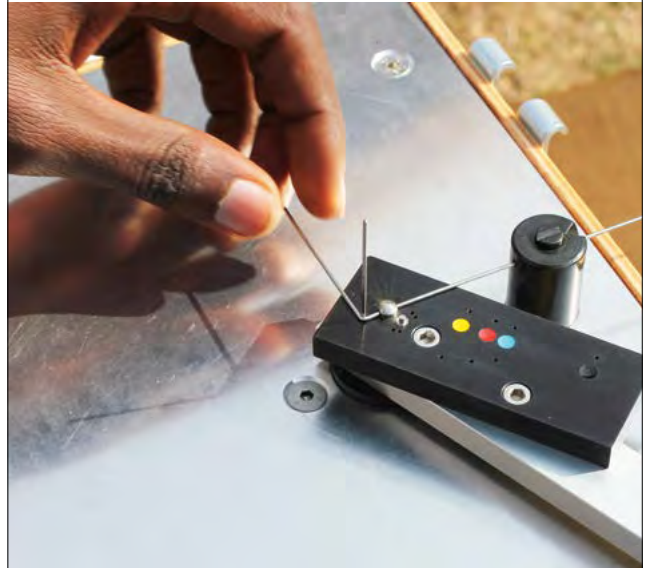
Color-coded markers, which refer to pupillary distance (PD), indicate different frame sizes (Yellow = small, Red = medium, Blue = large)
