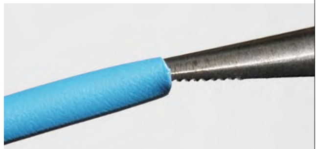
4 Tuck the cut end inside the new tubing
