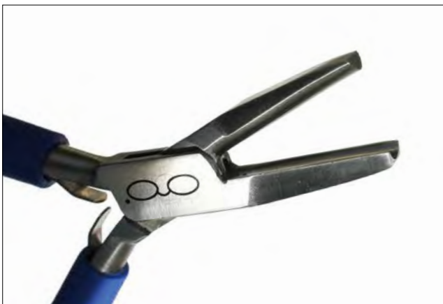
Loop-forming pliers—to shape the temple ends
