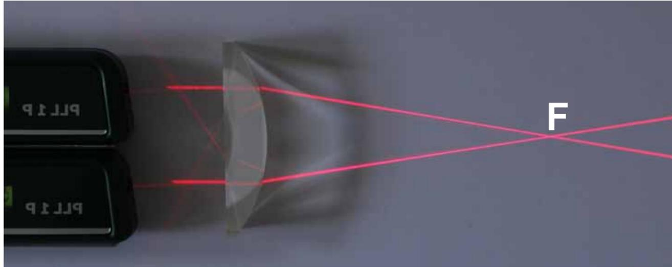
Positive lens – focuses the light rays in the focal point F
