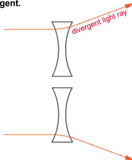
When many (millions) of light rays pass through the lens as a parallel light beam, all of them get refracted ...
