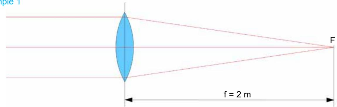
This lens has a focal length of  $f = 2 \text{ m}$
